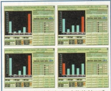
AIBB provides us with an Amiga showdown. And just look how well the 1230-II Turbo performed. In all tests it matched the A4000 and even beat it in the LineTest. With the addition of an FPU and the execution of FPU specific tests, expect to see your A1200 overpower the competition greatly
